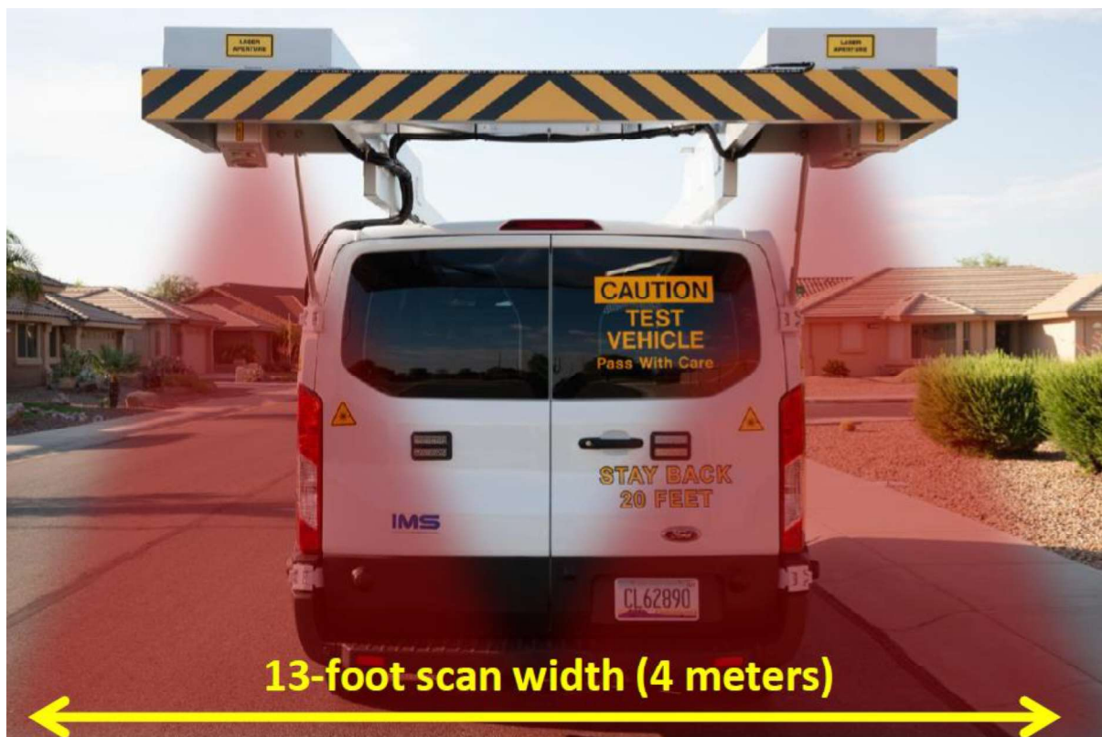
Figure 5 - RST Equipped with the 3D LCMS-2 Camera
